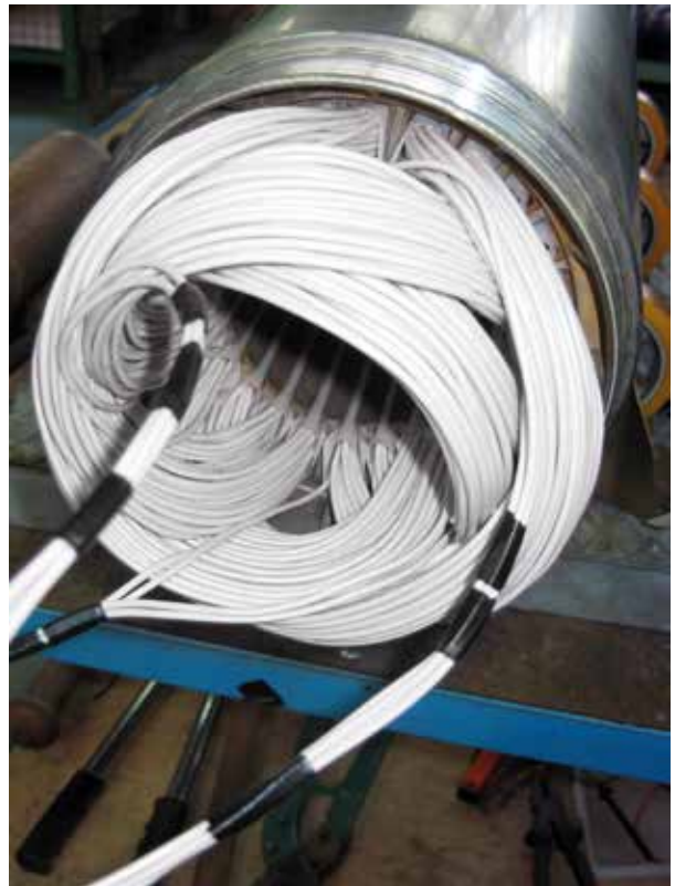
Automatic winding process for standard motors with PE-insulated winding wires.
