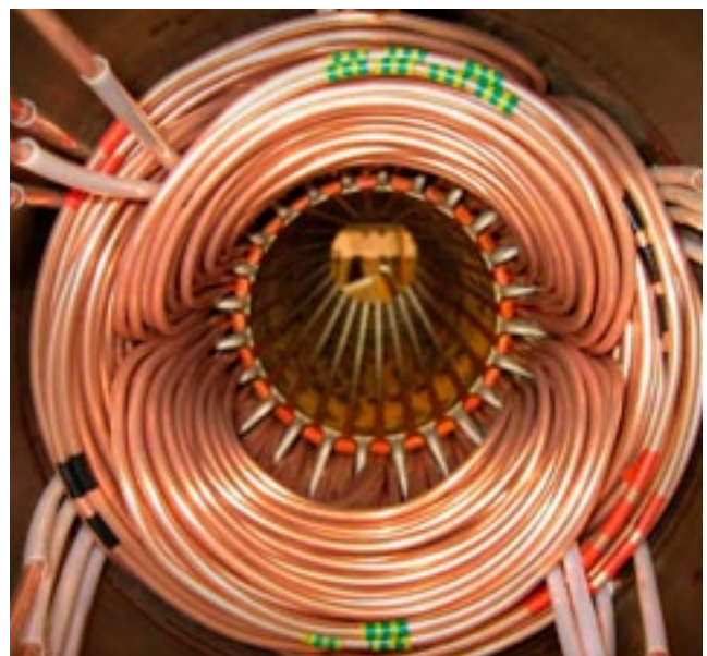
Motors for special applications with PE2/PA insulated winding wires
